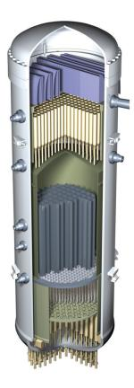
The ESBWR (Economic Simplified Boiling Water Reactor) builds on a long line of proven GEH BWR reactors. ESBWR employs passive safety design features. It is a simplified reactor design, allowing faster construction and lower operating costs.
